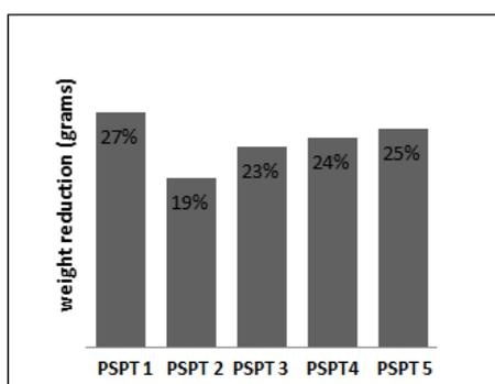
**Fig. 2. Average Weight Loss of PS-Starch Coating Polymer for 4 Weeks**
